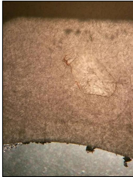
Injection Molded Plastic Component, machined down for FTIR identification of polymer inclusion.
