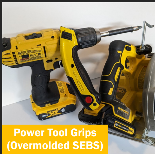
SBS/SEBS are commonly encountered in power tool grips, either alone or compounded with polyurethane. The high surface friction helps to avoid slipping.
